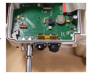
Pieces in which the pressure connections are screwed.
