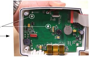
> Connect and clip the pressure board on the red connector and on the spacers previously put in place.
