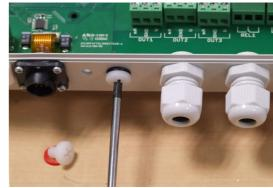
> Put the two pressure connections with the color rings and tighten them.
